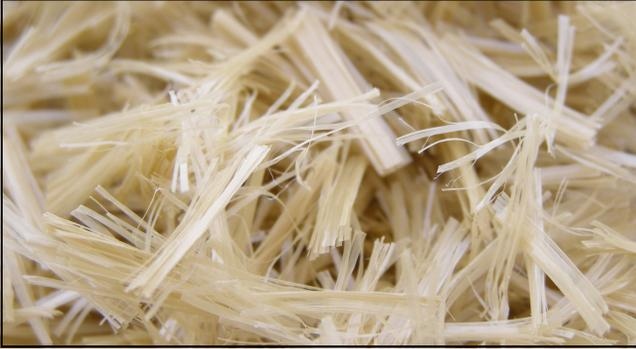
SportGrids are safe, non-toxic, polypropylene fibers, typically 1-2 inches long, fibrillated or tape polypropylene strands that are mixed or blended into sand or clay soils. During the blending process the fibers open or filamentize into net, grid and fiber configurations that mechanically reinforce any soil classification. This process creates a new soil structure with enhanced engineering properties that have been specifically designed to maximize shear strength.
